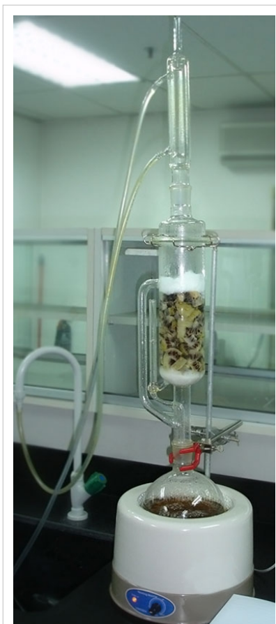
Fruit extraction in progress. The sample is placed in the thimble.
