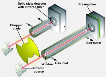
The lengths of the cells can be individually optimized, to obtain maximum precision for the target analysis levels of each customer. Each of the cells can be installed with infrared absorption lengths ranging between 1 mm and 320 mm.
